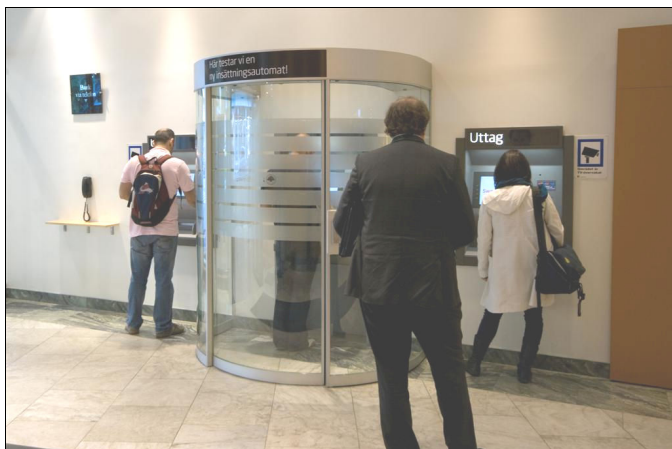
QCR with integrity booth surrounding the deposit area and two attached withdrawal fascias.
